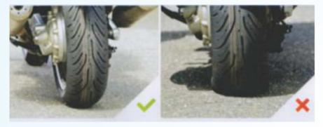
Always inflate the tyre to the correct pressure. Be sure to check cold inflation pressure frequently, i.e. once a week. Although most motorcyclists love to work on their bikes, they seldom remember to check tyre pressures. Correct tyre pressure, however, is critical for safe handling. Over inflation or extreme tyre pressure will impair your riding comfort and decrease the contact of the tyre with the road.
