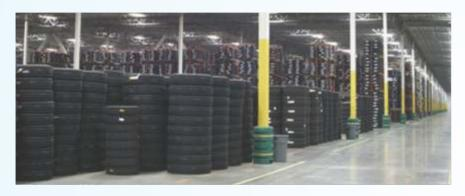
In bad weather conditions, unloading at the time of receipt must be carried out in a covered area; in any event, if water is found inside the tyres, this must be removed immediately. Unloading must not be carried out by dropping the tyres or by any other method which could damage the quality or visual aspect of the tyres. Tyres must not be moved by inserting the forks of a fork lift truck through the center of a tyre which could damage the bead area.
